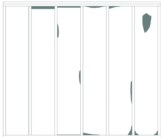
Figure 2 Grade I boundary condition: 2% compressed or incomplete fill area.
